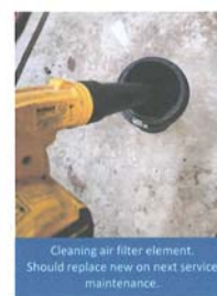
Air filter element cleaning
