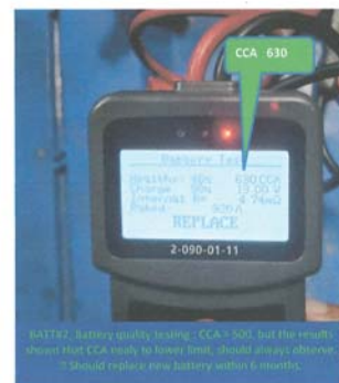
BATT01 Battery quality testing - CCA - 500, should replace new battery ***Should replace new battery***
